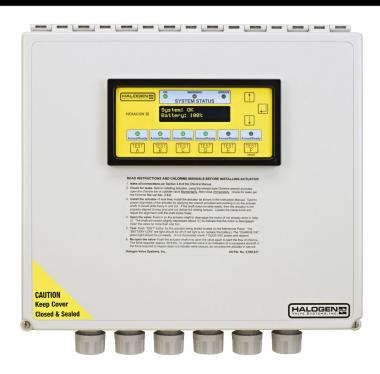
When used with our Eclipse actuators, the Hexacon III controller allows operators to remotely close up to six chlorine or sulfur dioxide valves in an emergency situation. The Hexacon III controller can interface with gas detectors, seismic or fire detectors, SCADA systems and with any number of remote mounted emergency shutoff/close switches. This allows operators to quickly and efficiently terminate a dangerous leak without having to "suit up" and enter the toxic environment.
